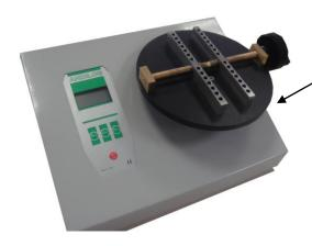
Mount the plate on the torque sensor
